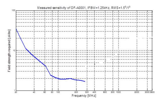
The graph illustrates the direction finding sensitivity of a typical system measured under specific electrical conditions. \*Note this is extracted from the DF-A0001 specification and only the performance of 20 to 300 MHz is applicable.
